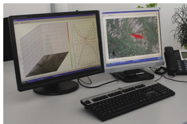
Impact analysis during a sounding rocket campaign. The picture shows the different results: on the left screen the nominal trajectory, altitude, Mach number and flightpath speed vs. time and on the right screen the impact footprint of a dispersion analysis.
